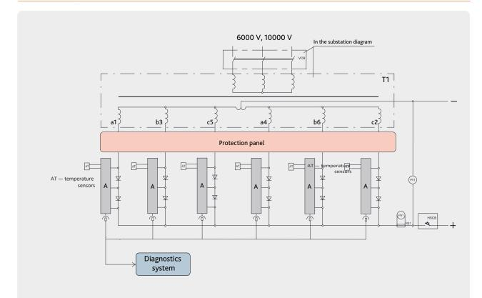
VCB — vacuum circuit breaker HSCB — high speed circuit breaker
