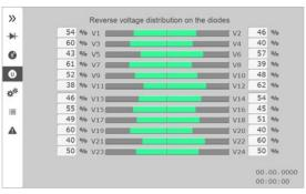
Information about state of the rectifier and its components is displayed on visualization panel, mobile devices (smartphone, tablet) or on the computer display via Web interface or special software.
